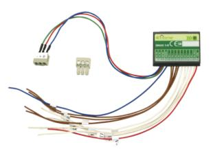
SimpleHome module with 5 digital inputs (4 normal + 1 scenario) for the connection of up to 5 buttons in flush-mounted or surface-mounted boxes. Dimensions: 41x29x9 mm. For connection to SimpleHome BUS. Consumption:
