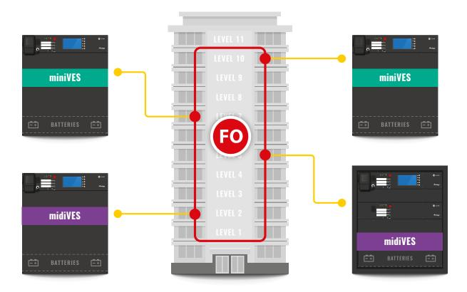
miniVES and midiVES are scalable Public Address & Voice Alarm units suitable for multi-purpose architectures. Devices from miniVES and midiVES series are voice alarm compact control units containing all components within one compact housing, which meet all the requirements of EN 54-16 and EN 54-4 (certificate of constancy of performance 1438-CPR-0527).
