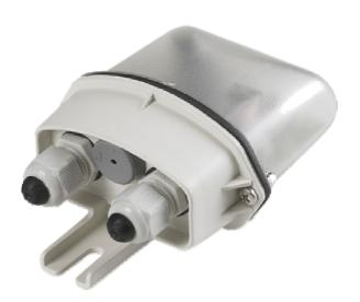
The CR2 photocell switch uses a photoelectric cell to automate ON and OFF controls on electrical appliances, according to the luminosity of its location. The switch threshold has a potentiometer adjustment; during this adjustment, the LED will light up to indicate the alignment between environment luminosity at that moment and the luminosity threshold setting.
