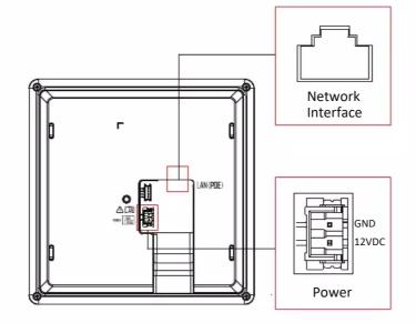
There is one network interface and one 12 VDC power interface on the rear panel of the indoor station.
