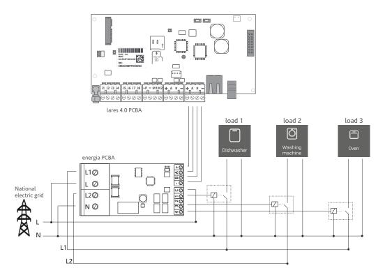
With reference to the diagram, it is possible to display the dishwasher and oven consumptions on line L1 and the washing machine consumption on line L2, on user App lares 4.0.
