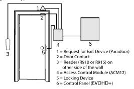
Persons authorized to access the protected area are issued cards assigned to user access codes programmed with an Access Level (see section) and a Schedule (see section). The control panel determines whether or not to unlock the door depending on the card's schedule and access.
