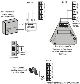
**NOTE:** If a door contact is not being used, install a jumper or a 1kOhm resistor across the blk and z1 terminals depending on the control panel's EOL definition. If the REX (Request for Exit) device is not being used, place a jumper across the blk and z2 terminals.
