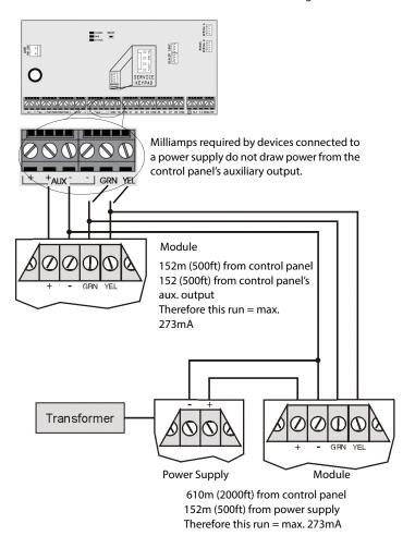
Figure 7: External Power Supply Connections
