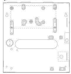
Installation of TK278 tamper kit (use single screw to attach bracket to wall)
