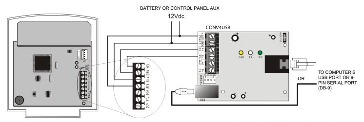
**NOTE:** K641, K641+, and K641R keypads that feature a four-pin serial connector can also be upgraded using the 307USB. To do this, the keypad's GRN and YEL Digiplex bus wires must first be disconnected.
