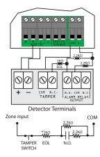
† Enable ATZ (see section on page 21) and connect as follows (extra input cannot be used)
