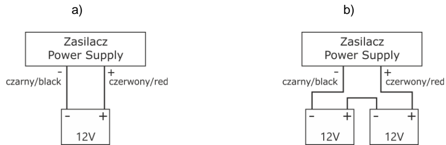
Fig. 4. Connecting batteries depending on voltage version of power supply: a) power supplies 12V version, b) power supplies 24V version
