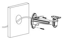
4 Fix the camera onto the base and screw up
