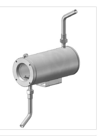
The optional BAX flange for glass cleaning creates an air barrier on the glass front of the housing in order to prevent the deposit of dust on the outer surface of the glass by keeping it ventilated.
