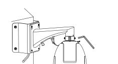
④ Fix the speed dome with set screw; installation complete
