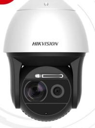
Hikvision Laser smart PTZ Dome Cameras DS-2DF8236I5W-AELW are able to capture high quality images in dim light environment with its laser IR light, which can reach up to 500m IR distance. Embedded with 1/1.9" progressive scan CMOS chip makes DWDR and 2MP real-time resolution possible. With the 36X optical zoom Day/Night lens, the camera offers more details over expansive areas.
