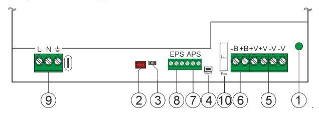
Fig. 2c. View of power supply module (12V20A, 24V10A models)
