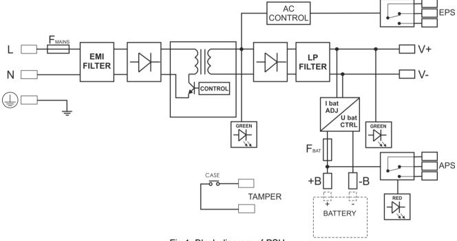
Fig.1. Block diagram of PSU.
