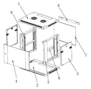
1 Top cover 2 Bottom cover 3 Frames Front door 4 5 Side panels 6 L- shape brackets 7 Rear panel Mounting bracket 8 9 Vertical brackets
