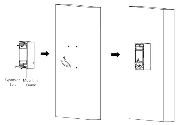
Figure 3-3 Fix the Mounting Frame
