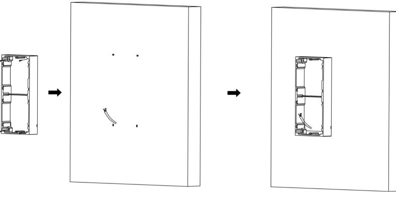
Figure 3-14 Fix the Mounting Frame
