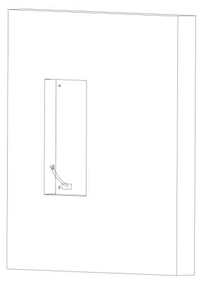
Figure 3-19 Drill the Installation Hole
