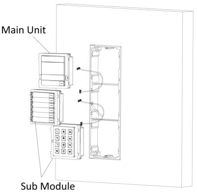
**Figure 3-35 Connect Cables and Insert Modules**
