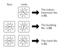
Figure 7-4 Example: DIP Switch of Indoor Station
