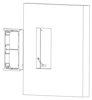
Figure 3-20 Fix the Mounting Frame
