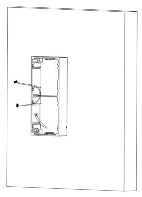
Figure 3-15 Placement of Lines
