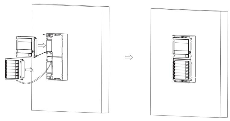
Figure 3-17 Insert the Modules
