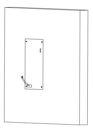
Figure 3-13 Drill Screw Holes
