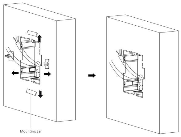
**Figure 3-9 Remove the Mounting Ears**
