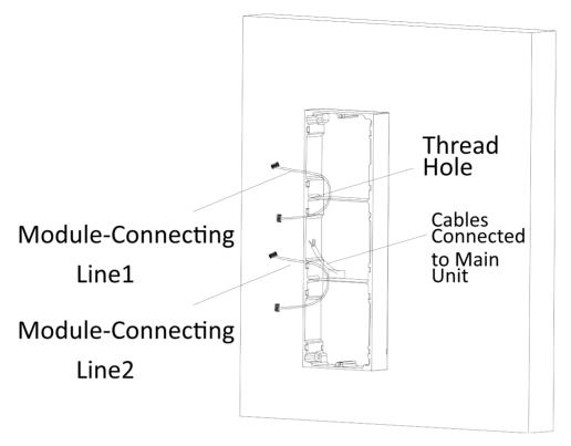
Figure 3-28 Connect the Cables
