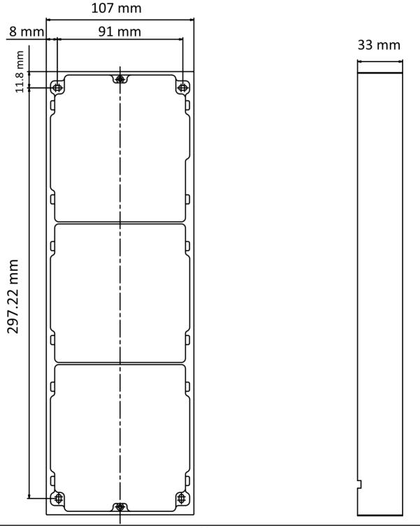
Figure 3-24 Mounting Frame
