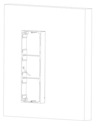
Figure 3-26 Fix the Mounting Frame
