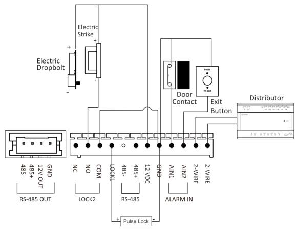
Figure 2-2 Wiring of Door Station
