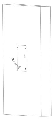
**Figure 3-2 Drill Screw Holes**
