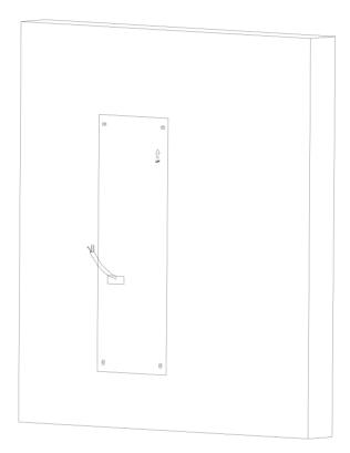
Figure 3-25 Drill Screw Holes
