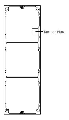
Figure 3-27 Mounting Frame
