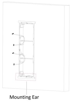
Figure 3-34 Remove the Mounting Ears
