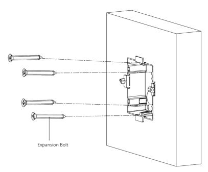
Figure 3-8 Fix the Mounting Fame
