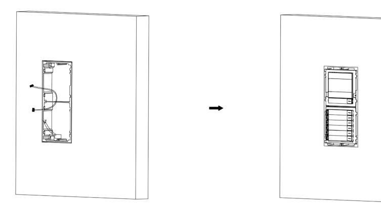
Figure 3-22 Connect Cables and Insert the Modules
