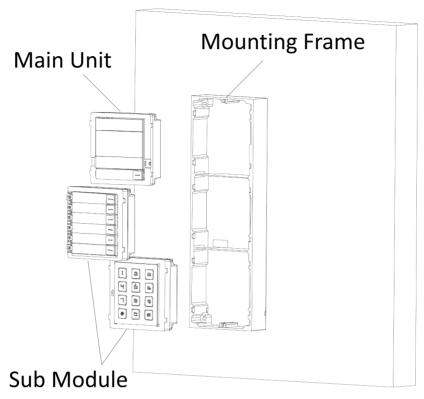
Figure 3-30 Insert the Modules into the Frame
