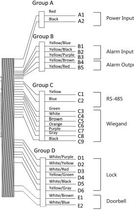
Figure 4-1 Terminal Diagram
