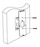
Figure 5-2 Install Mounting Plate
