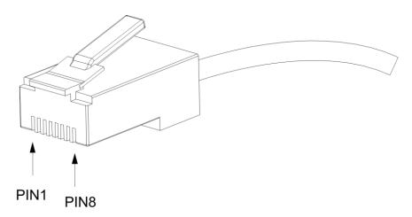
Figure 3-7 RJ-45 connector of the console port
