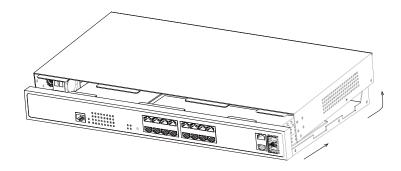
When the cover is opened, put it aside. The main board of the system appears.
