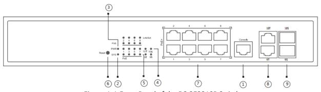
Figure 1-1 Front Panel of the DS-3E2310P Switch
