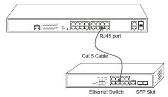
Figure 3-8 Connecting Base-T ports and other Ethernet terminal
