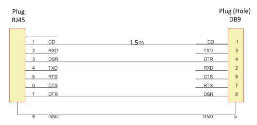
Figure 3-5 Cable connection at the console port
