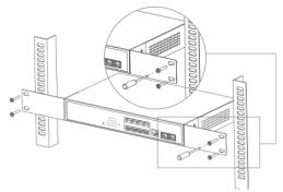
Figure 3-2 Installing the switch on the cabinet
