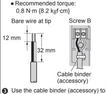
secure the DC cable (double-coated area) to the main monitor
