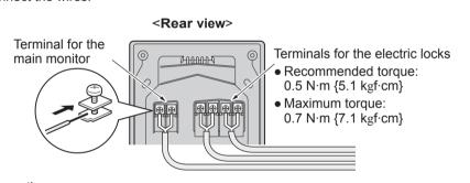
**3-2** Push in the wires to the terminal connectors (non-polar), then tighten the screws.
