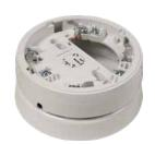
The sounder consists of a white plastic housing and is designed for indoor ceiling mounting. The integrated detector base accommodates an automatic detector Series FI750. The loop address is set in the range 1 to 240 by means of the Programming Unit FI750/PU. Furthermore, in case of connection to a compatible fire detection control panel, the sounder can also be AUTO-addressed. If a short circuit occurs on the loop line, the integrated dual-isolator will disconnect the loop.
