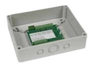
The module occupies 8 consecutive addresses on the loop. The base address is set in the range 1 to 240 by means of the Programming Unit FI750/PU. Furthermore, in case of connection to a compatible fire detection control panel, the module can also be AUTO-addressed. If a short circuit occurs on the loop line, the integrated dual-isolator will disconnect the loop.
