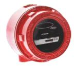
The response delay can be set by selecting one of four values between 1 and 8 s. The alarm and the fault condition are signalled via two dry relay contacts. The functioning of the detector can be checked by means of the integrated self test function. Here the detector is activated by a built-in source of infrared light.
