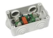
The line coupler is integrated in a grey plastic housing and is designed for indoor surface mounting.
