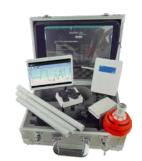
interface. The tablet graphically displays the field strength of the connection between the wireless devices. If the field strength is too low, the location of the RF components must be changed. The readings are updated continuously.
