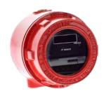
The response delay can be set by selecting one of four values between 1 and 8 s. The alarm and the fault condition are signalled via two dry relay contacts. The functioning of the detector can be checked by means of the integrated self test function. Here the detector is activated by a built-in source of infrared light.
