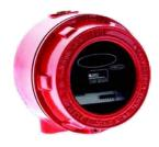
The response delay can be set by selecting one of four values between 1 and 8 s. The alarm and the fault condition are signalled via two dry relay contacts. The functioning of the detector can be checked by means of the integrated self test function. Here the detector is activated by a built-in source of infrared and UV light.
