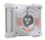
The detector has 4 sensitivity ranges that can be selected by the user. For each range there are 2 response levels. The response delay of the detector can be set to one of four values between 5 and 10 s. An alarm and a fault condition is signalled via two dry relay contacts. Conventional technology is used for alarm transmission to the fire detection control panel. Integration into a loop can be achieved by means of a conventional zone module.
