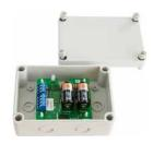
Two batteries are accommodated in the housing of the module. Normally, the module is powered by the main battery. In the event of a failure of the main battery, the secondary battery powers the module. The two-coloured LED indicates the activated condition and the fault condition of the module.
