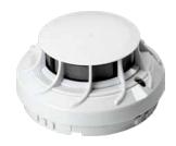
set through the fire detection control panel to one of nine levels between 0.03 %/m and 3.3 %/m, depending on the detection task. An optional pre-alarm can be activated two levels before reaching the alarm threshold.
